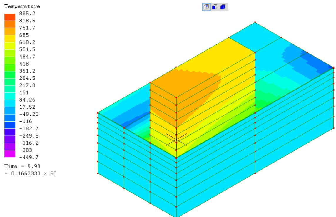
Figur 1. Temperature distribution in a fired zirconia-porcelain strip 10 seconds after placement on the enamelled cooling plate.
