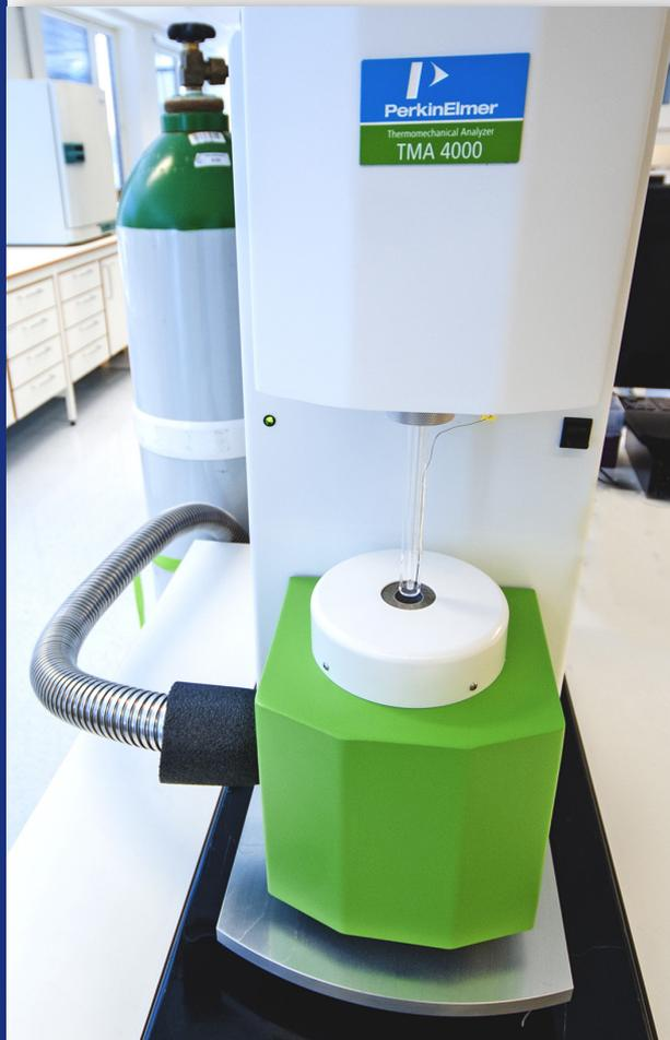
Thermomechanical analysis provides valuable insight into structural changes or phase transformations. Coefficients of thermal expansion for the core material and the veneering material will always be different and stresses will be built up between the two materials by repeated heating and cooling during veneering.
