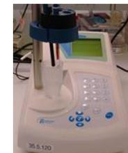
Figure 3: Fluoride measurement equipment.
