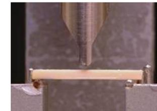
Figure 2: GI-specimen in three-point bending test.
