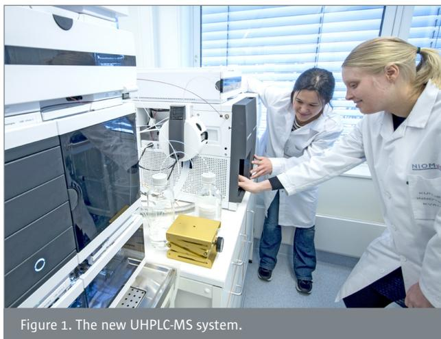
Figure 1. The new UHPLC-MS system.
